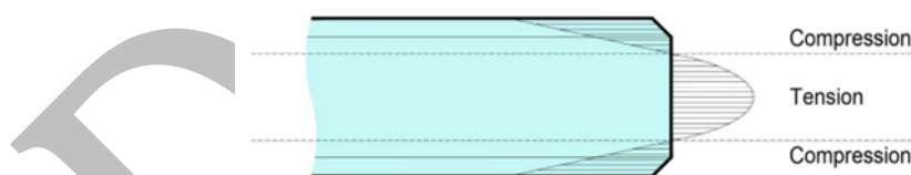
Figure 2 – Stress profile in tempered glass
